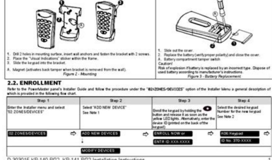
1. Drill 2 holes in mounting surface, insert wall anchors and tighten the bracket with 2 screws.
